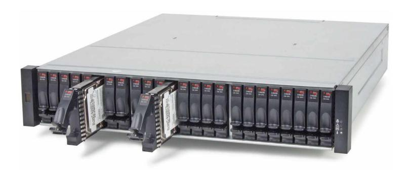
"[...] is a data storage virtualization technology that combines multiple physical disk drive components into one or more logical units for the purposes of data redundancy, performance improvement, or both."
